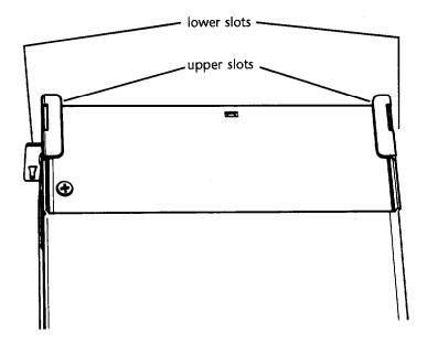
There are four corresponding tabs on the inside back panel of the computer which fit into the openings in the subassembly slots.
